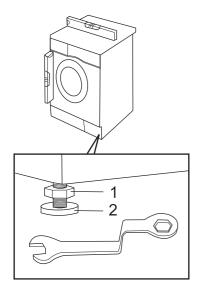
By adjusting height of the machine legs, and by gradienter, adjust the levelness of the machine.
